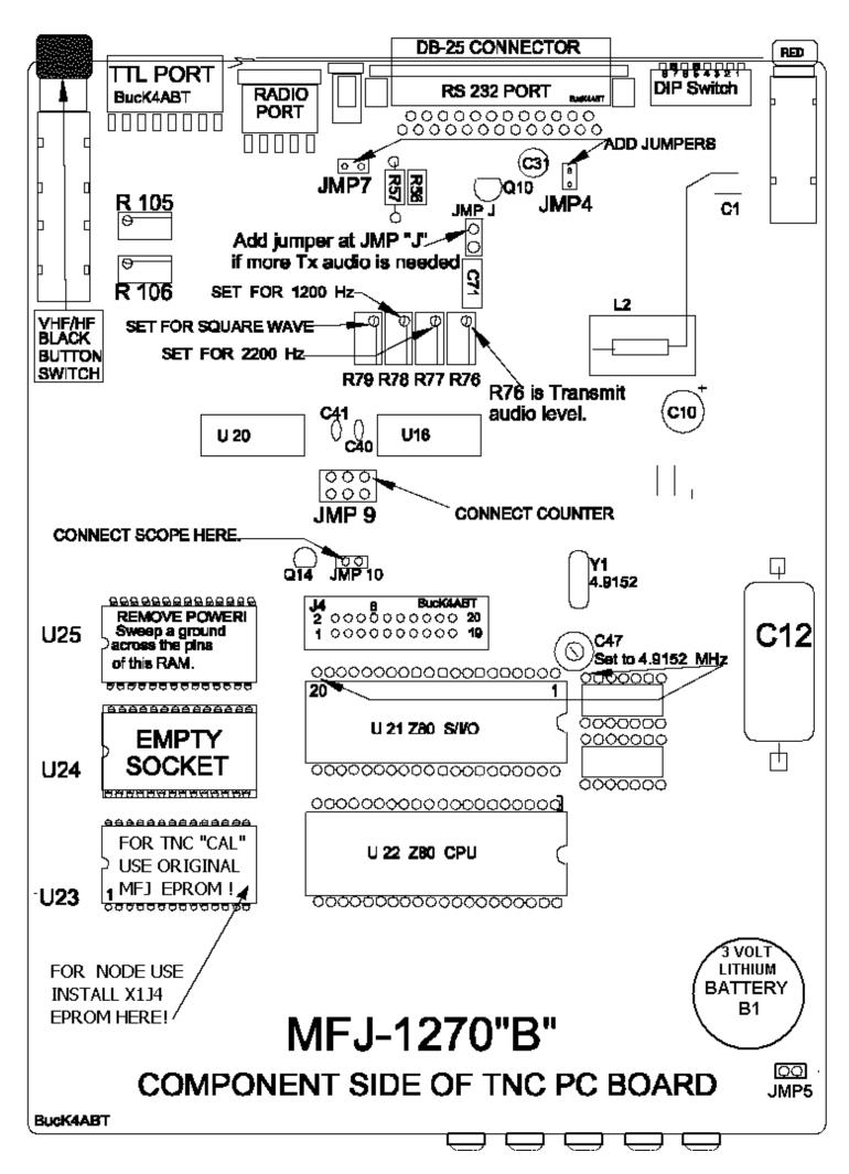
1- Power ON. Connect Frequency counter to U21, pin 20, set C47 to 4.915205
