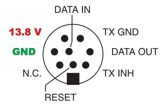
NOTE1: This connector has two operating modes selected by moving a jumper inside the radio. In the default mode shown on this diagram, the connector is a serial data port for computer interface. The alternate mode uses this connector for hardware-based band selection on a companion Yaesu linear amplifier.
