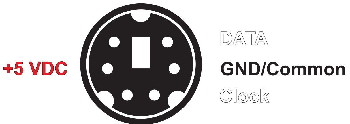
Looking into Female Jack (Soldering end of Male Plug)
